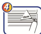
4 Spray Mr McKenic®-Air Conditioner Cleaner ~10cm away from the fins in a S-motion from top to bottom. Allow 15-20mins for product to penetrate into the interior.
