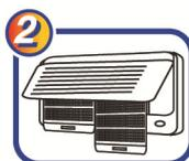
2 Open casing to remove dirty filters for washing. Use a vacuum cleaner or brush to remove thick layer of dust from cooling fins, if applicable.
